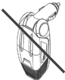
1. Do not position the unit downward (as shown in the diagram at the left). Doing so will subject the unit to discoloration and irreparable damage.
